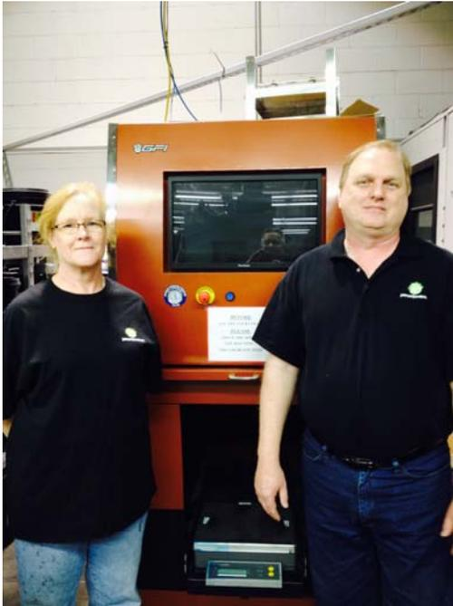
*J/A production manager Phil Huxhold and production assistant Deb Hara with the firm's AccuBlend-LV water-flexo ink dispenser. While generating ink colors precisely to spec when and as needed, the dispenser has virtually eliminated press run delays and job switching, and reduced press prep time by about 20 minutes per job.*
